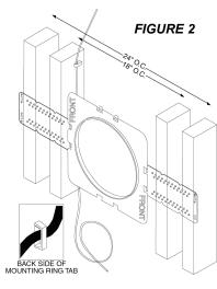
Step 2. After you determined have the speaker locations using the guidelines above. secure a 16 gauge 2 - conductor cable to the mounting ring tabs (see figure 2), such as the M&S Systems MS16X, for attachment to the speakers after the dry wall has been
